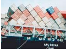
> Up to 10,000 containers are lost annually due to extreme rolling
