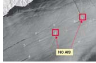
> Ship detection by assimilation of Earth Observation and Automatic Identification System (AIS) data
